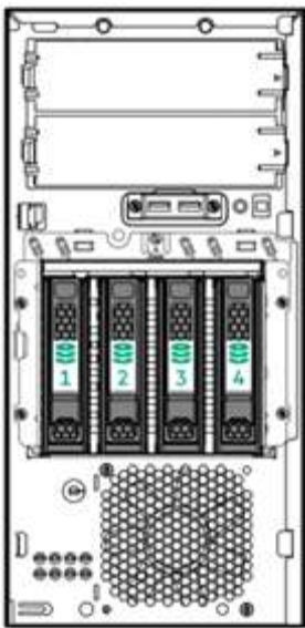
4 LFF Hot-Plug Drive Model 1-4 4 x LFF SAS/SATA/SSD hot pluggable hard drive bays
