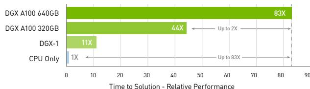
Big data analytics benchmark | 30 analytical retail queries, ETL, ML, NLP on 10TB dataset | CPU: 19x Intel Xeon Gold 6252 2.10 GHz, Hadoop | 16x DGX-1 (8x V100 32GB each), RAPIDS/Dask | 12x DGX A100 320GB and 6x DGX A100 640GB, RAPIDS/Dask/BlazingSQL. Speedups normalized to number of GPUs.
