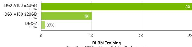
DLRM on HugeCTR framework, precision = FP16 | 1x DGX A100 640GB batch size = 48 | 2x DGX A100 320GB batch size = 32 | 1x DGX-2 [16x V100 32GB] batch size = 32. Speedups normalized to number of GPUs.
